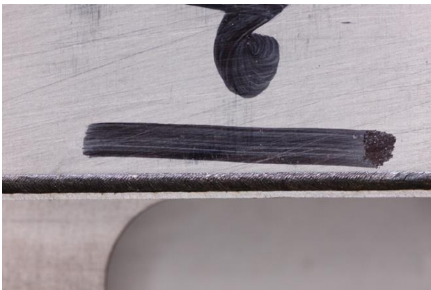
Figure 4.1 – Image of welded Package, circular weld path
